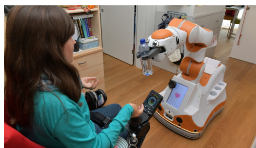
Envisioned approach 2: A person in a powered wheelchair and a robotic manipulator mounted to an auxiliary mobile platform. Image source
